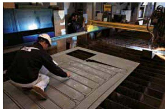
All CRN hulls are built in steel with the plates CNC cut on site. The superstructures are all aluminium
