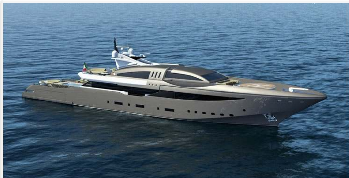
CRN's 62-meter Dislopen design shows open-deck characteristics atop an efficient displacement hull. Cruising speeds will be about 14 knots. Note the helipad forward.
